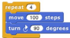
That's a trick question; the *move* block is run four times, and it has a different continuation each time. The first time, its continuation is
